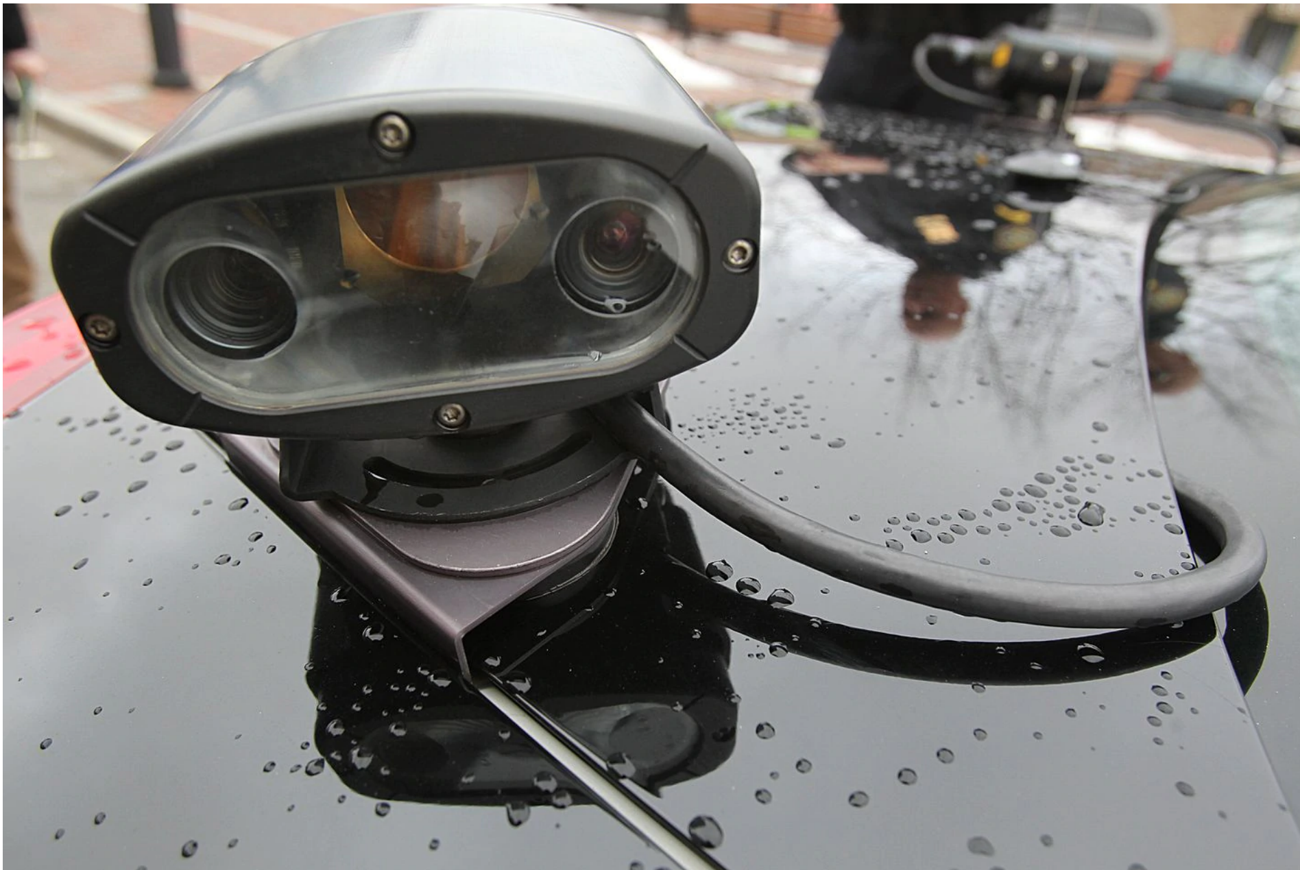
An automatic license plate reader atop a police car. SUZANNE KREITER/GLOBE STAFF/FILE 2013/GLOBE STAFF
